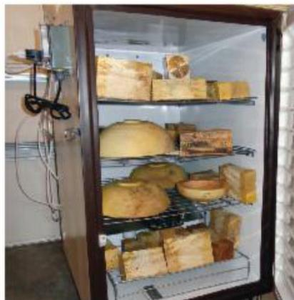
regulates the temperature inside the kiln by automatically turning the bulbs on or off so that a consistent temperature is maintained. I drilled four 1/2" (13mm) holes in the bottom of the freezer below the lightbulbs and four matching holes in the upper rear wall. Heat convection from the bulbs draws outside air into the freezer through the bottom holes. Warm humid air exits the freezer through the top holes.
