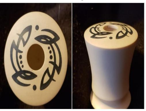
Started a new turned hollow container made from Holly. I used my laser to cut a design into the top and used black milliput epoxy to fill it in. The design ended up being a little smaller on the top than I like but I really like the look of the crispness of the design done with the laser. I'm still trying to decide on what to do for the lid. The piece is about 1 1/2" high.
